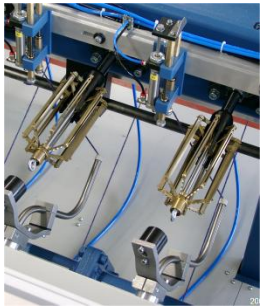
Automatic winding with doffing device and optional cup conveyor belt
