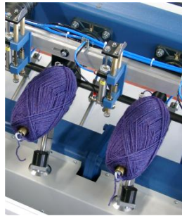
Automatic winding with doffing device and optional cup conveyor belt
