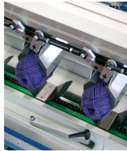
Servo drive, automatic yarn cutting device
