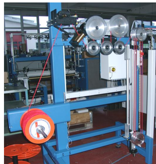
Supply creel with knot detection device and dancer
