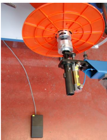
Spool clamping device, activated with foot switch (option)
