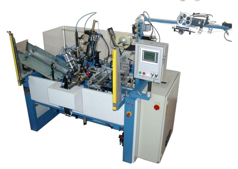
Ribbon and rope precision winding and rolling machine BS 1 - PW and BSH - PW
