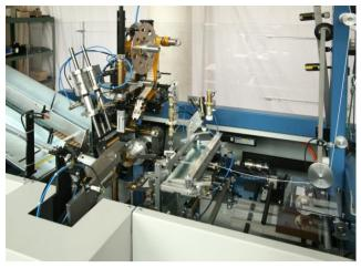
Semi automatic universal machine BSH-PW for spooling and rolling of textile and plastic ribbon and rope on cardboard or plastic cores with or without side flanges.
