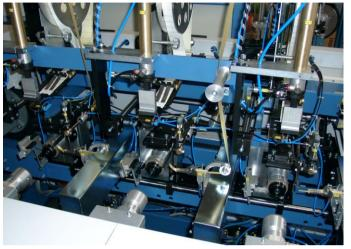
cups on the same cup conveyor. The cup conveyor indexes forward and empty cores are lifted into winding position. The winding mandrels clamp the empty cores between two friction discs. The ribbon guiding system moves towards the empty core and the ribbon is attached to the core with an adhesive label.
