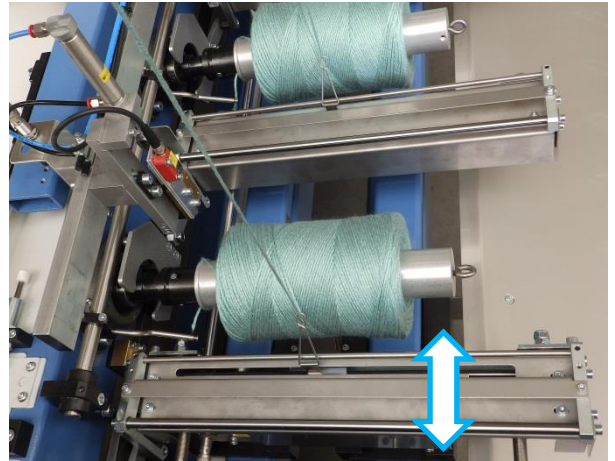
Gliding traverse system for constant distance
