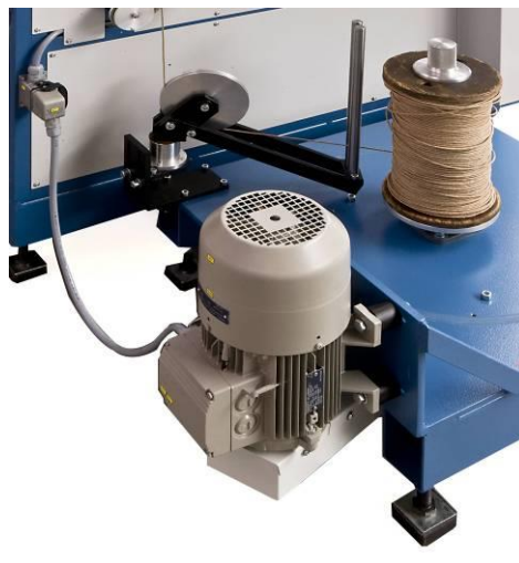
Inverter controlled creel drive of supply package for constant winding speed and yarn tension.
