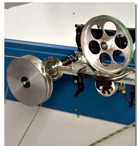
Length measuring device and yarn brake (standard delivery with creel).
