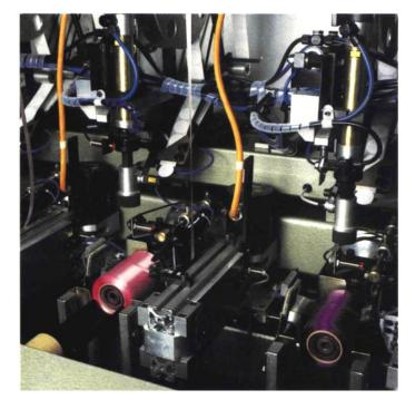
winding cycle tubes are released out of the magazine and transported to each winding position with a cup conveyor. After the previous winding cycle is finished, the empty tubes are pushed onto the mandrel of each winding position. The ribbon guiding system moves towards the empty tube and the ribbon is attached to the tube with an adhesive label.
