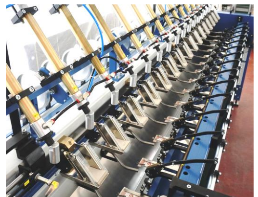
Card magazine above each winding position
