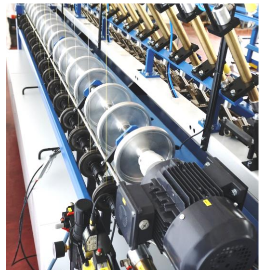
Active yarn delivery device, adjustable
