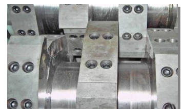
Segment knives, can be exchanged without dismantling of the cutting shafts
