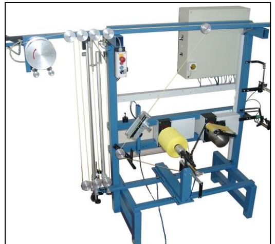
Combination creel for supply spools and to pull out of boxes
