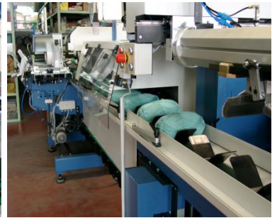
Servo drive, automatic yarn cutting device
