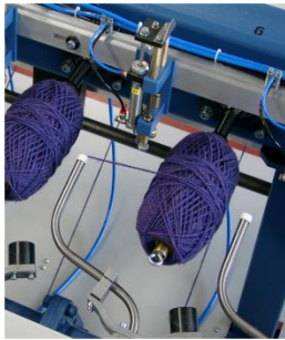
Automatic winding with doffing device and optional cup conveyor belt
