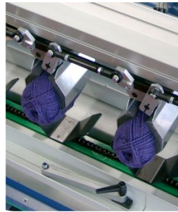
Servo drive, automatic yarn cutting device
